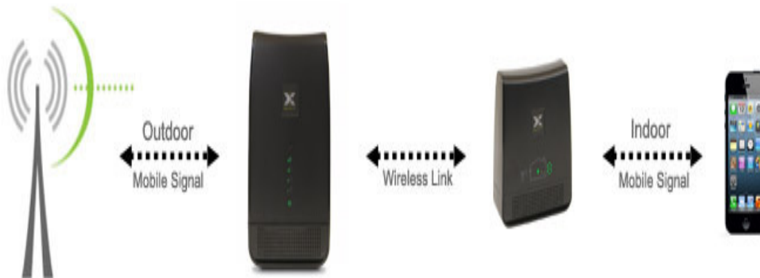
Figure-1 How 3G works with mobile phone
